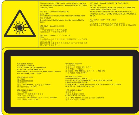
Laser warning label is located at the rear side of the projector as shown in the illustration below.
